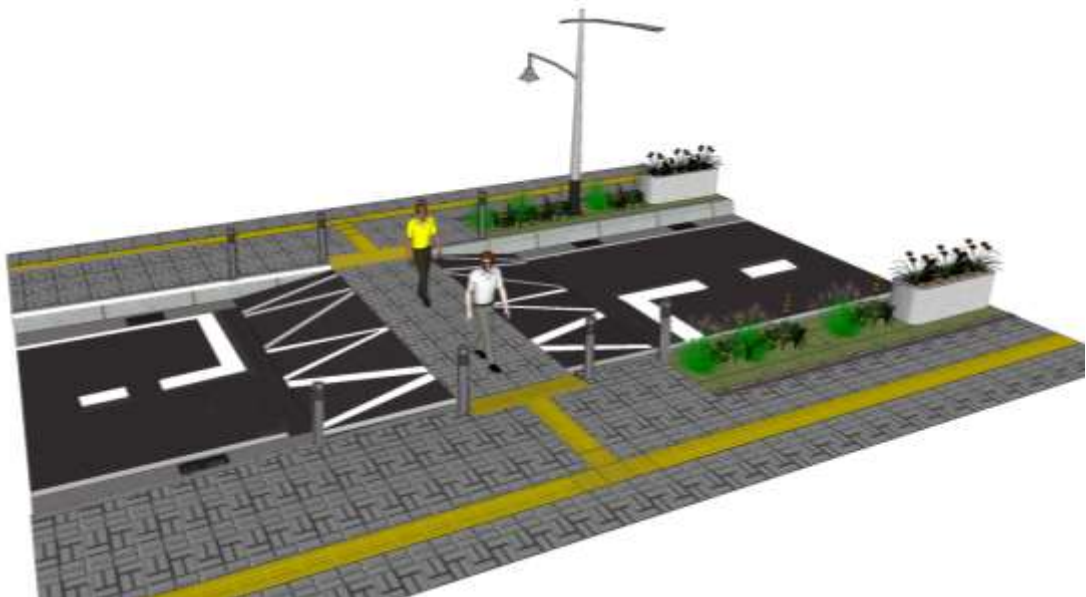
Gambar 9 - Contoh pedestrian platform di ruas jalan
