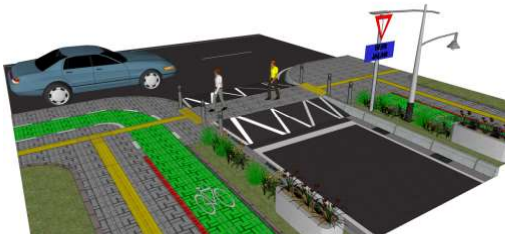
Gambar 10 - Contoh pedestrian platform di persimpangan
